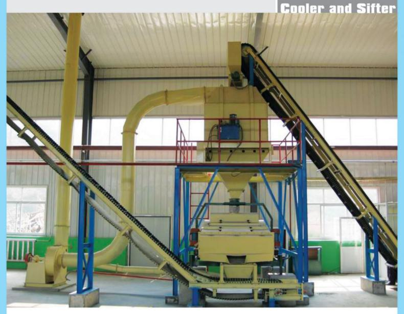
After the pelletizing process, the temperature of the wood pellet is about 60-80 degree Centigrade, and the moisture content of the wood pellet is about 15%. So we need to use a cooler to reduce about 3-4% of the moisture, which makes the wood pellet easy to store
